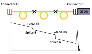
Figure 96. OTDR measurement from connector E to connector O (E->O)
