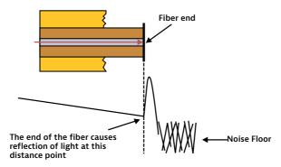
Figure 100. Break or fiber end location
