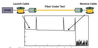
Figure 99. Acceptance testing using launch and receive cables
