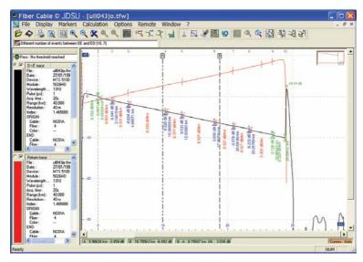
Figure 105. Bidirectional analysis using VIAVI FiberCable software
