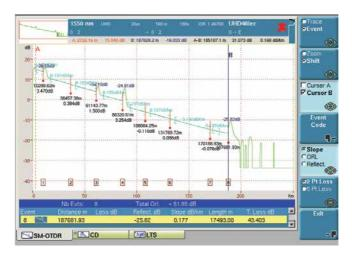
Figure 73. Automatic event detection using the VIAVI T-BERD/MTS platforms
