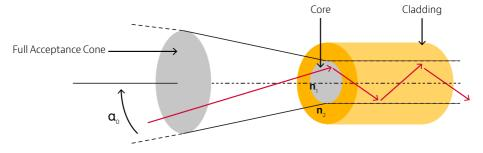
Figure 2. The injection of light into a fiber
