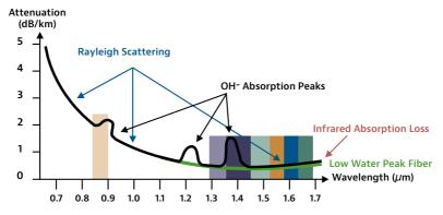
Figure 15. Fiber attenuation as a function of wavelength
