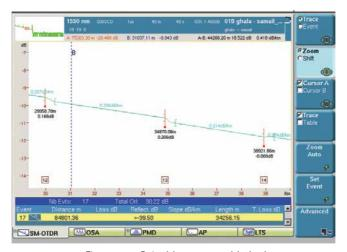
Figure 79. 5-Point Measurement Method
