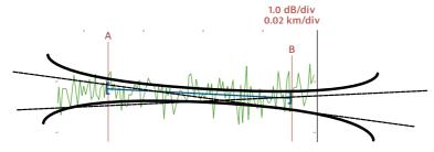
Figure 76. Using the 2-point measurement method between cursors A and B
