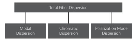
Figure 19. Types of fiber dispersion
