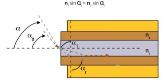
Figure 3. Refraction of light
