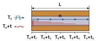
Figure 55. The OTDR pulse generation principle
