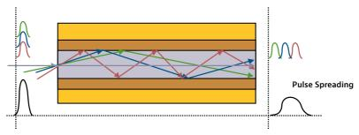
Figure 20. Modal dispersion in step-index multimode fiber
