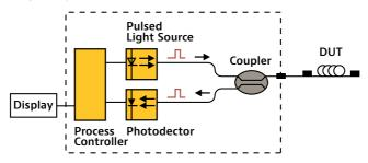
Figure 35. Setup using the OTDR method
