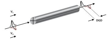
Figure 22. Polarization mode dispersion (or differential group delay) effects on a fiber
