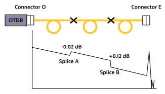
Figure 95. OTDR measurement from connector O to connector E (O->E)
