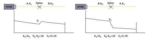
Figure 89. A positive splice A to B
