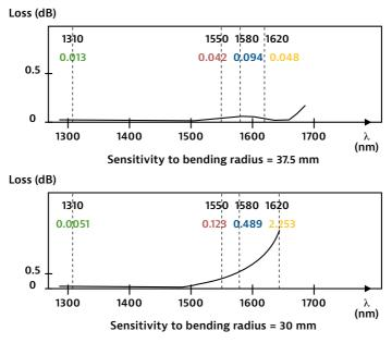
Figure 64. The effects of bending on a fiber
