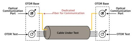
Figure 102. Automatic bidirectional OTDR measurement configuration
