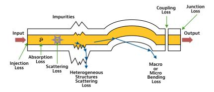
Figure 16. Link loss mechanisms
