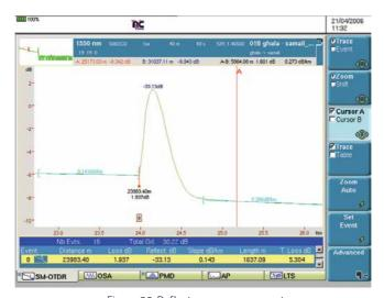
Figure 80. Reflectance measurement
