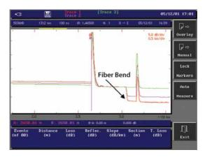
Figure 65. The OTDR graph shows a bend located at 3040 m at 1550 nm and 1625 nm
