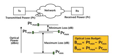
Figure 32. Calculating the optical loss budget
