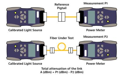
Figure 28. The insertion loss method uses two steps to measure the attenuation along a fiber link
