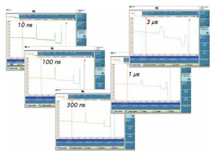
Figure 67. Fiber measurement using different pulsewidths
