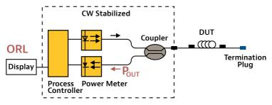
Figure 34. ORL measurement using the OCWR method
