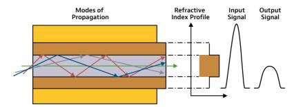
Figure 9. Light propagation through step-index multimode fiber
