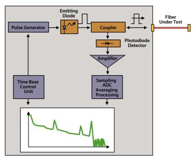
Figure 48. A schematic diagram showing OTDR technology
