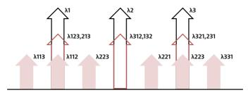
Figure 24. Four wave mixing of a signal on a fiber
