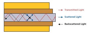
Figure 14. Backscattering effects of light transmission
