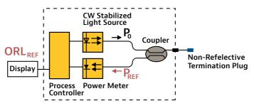
Figure 33. ORL referencing using the OCWR method
