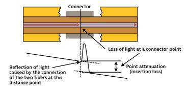
Figure 69. A reflective event at a connector junction
