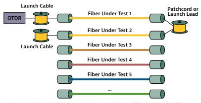
Figure 103. A loopback measurement, measuring O->E of fiber 1 and E->O of fiber 2
