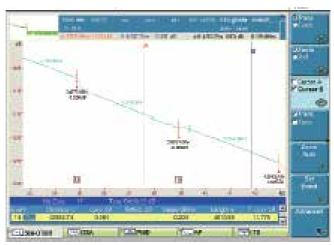
Figure 87. A splice gain on an OTDR trace
