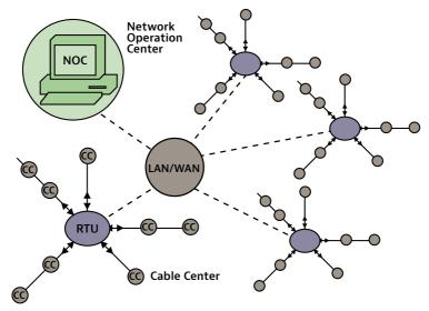
Figure 42. A remote monitoring system
