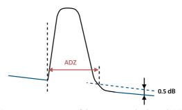
Figure 59. Measurement of the attenuation dead zone (ADZ)
