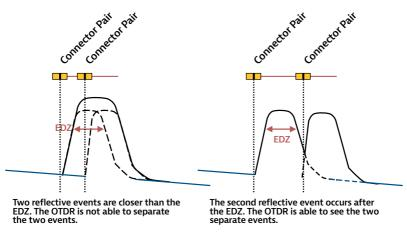
Figure 63. Event dead zone and connector discrimination by the OTDR
