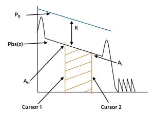
Figure 83. Section ORL measurement
