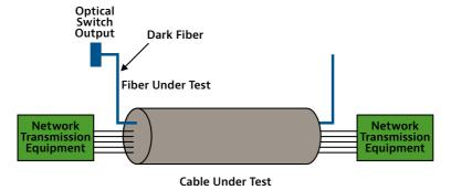
Figure 43. Out-of-service monitoring of a link
