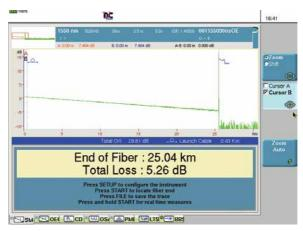
Figure 101. Fault location usiing an OTDR
