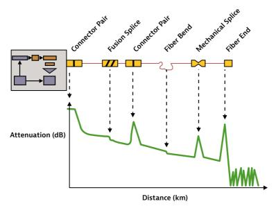
Figure 56. A typical OTDR trace
