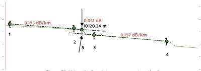
Figure 78. Using the 5-point measurement method
