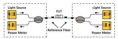
Figure 29. Insertion loss measurement with two bi-directional loss test sets
