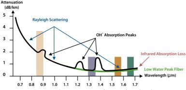
Figure 46. Fiber attenuation as a function of wavelength
