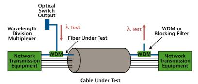
Figure 44. In-service monitoring of a link
