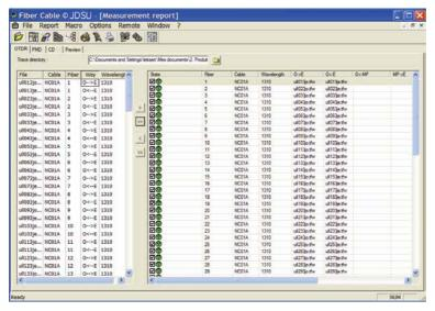
Figure 106. The template is applied to all the fibers using VIAVI FiberCable software
