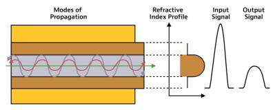
Figure 10. Light propagation through graded-index multimode fiber
