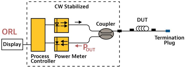
Figure 34. ORL measurement using the OCWR method
