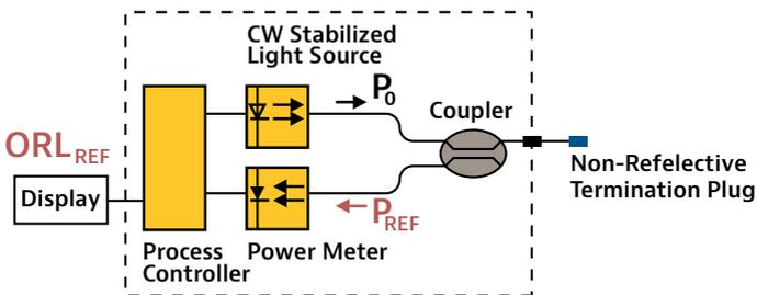
Figure 33. ORL referencing using the OCWR method
