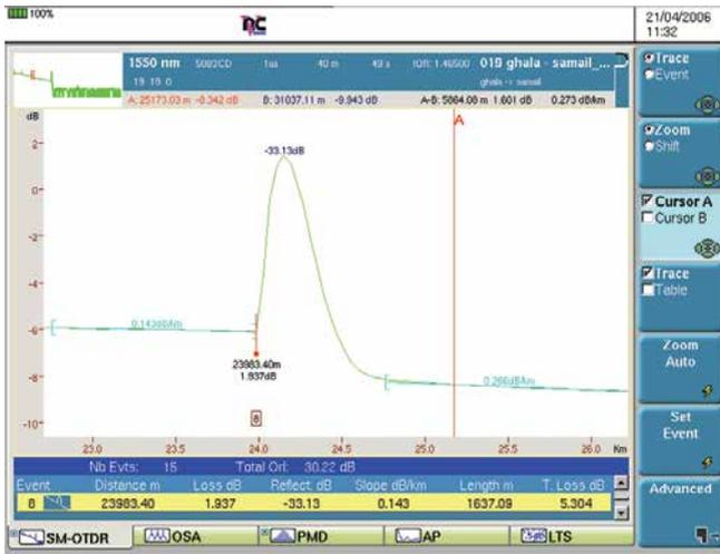
Figure 80. Reflectance measurement
