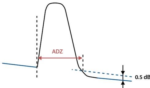
Figure 59. Measurement of the attenuation dead zone (ADZ)
