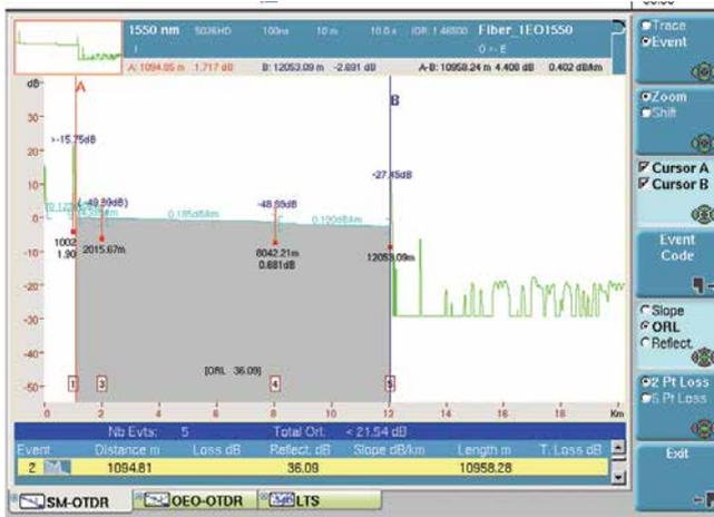
Figure 81. ORL measurement of a fiber link
