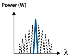
Figure 51. The emitted spectrum of a DFB laser
