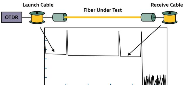
Figure 99. Acceptance testing using launch and receive cables
