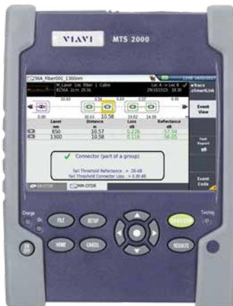
Figure 36. VIAVI T-BERD/MTS-2000 Mini-OTDR test instrument
