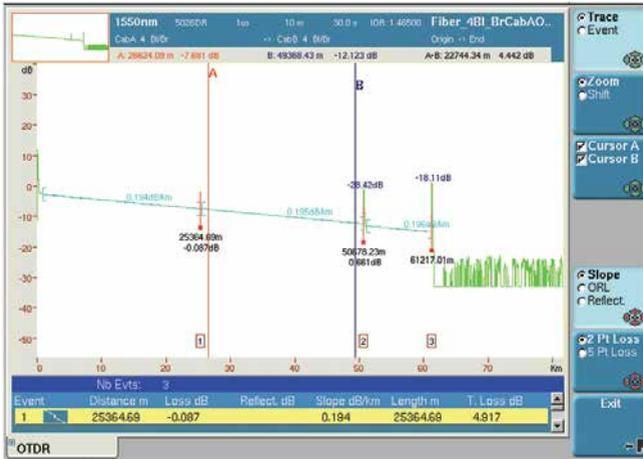
Figure 75. Manual measurement using cursors A and B
