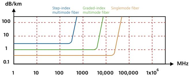
Figure 6. Typical bandwidths for different types of fiber
