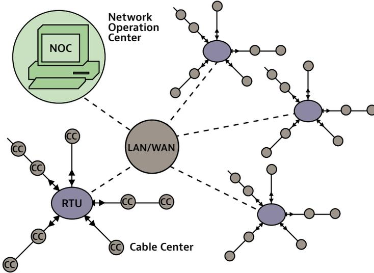
Figure 42. A remote monitoring system
