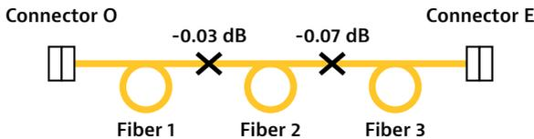
Figure 94. Actual fusion splice loss
