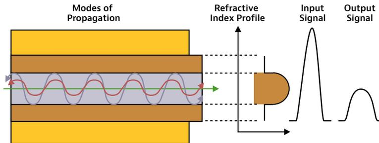
Figure 10. Light propagation through graded-index multimode fiber
