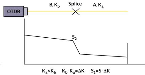
Figure 90. A negative splice from B to A
