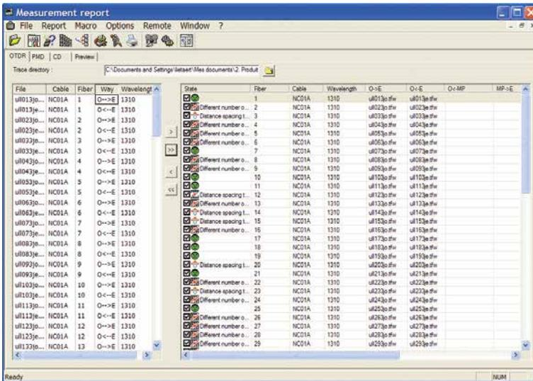
Figure 104. Test results management using VIAVI FiberCable software
