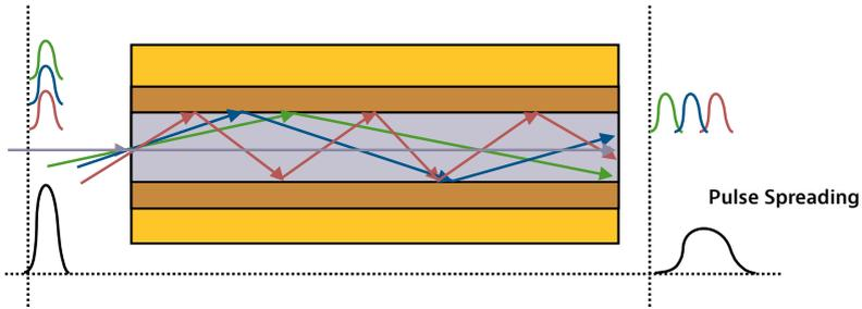
Figure 20. Modal dispersion in step-index multimode fiber
