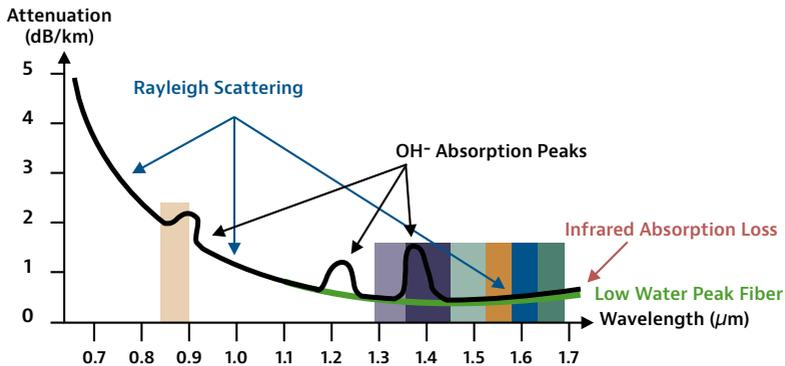
Figure 15. Fiber attenuation as a function of wavelength
