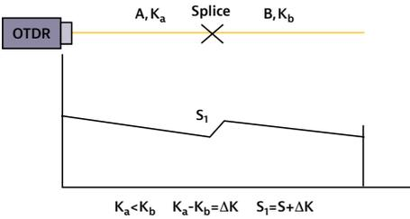
Figure 89. A positive splice A to B
