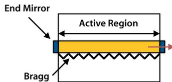
Figure 52. A schematic diagram of a DFB laser
