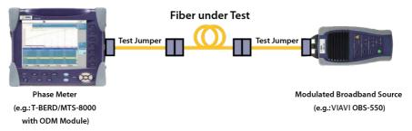
Figure 84. CD test setup with the VIAVI solution
