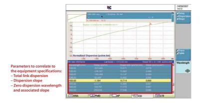
Figure 85. CD results with the VIAVI Phase Shift method (ODM module)
