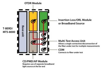
Figure 91. Schematic of the T-BERD/MTS-8000 MTAU and the accociated plug-in module connections
