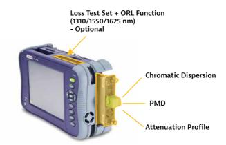
Figure 67. VIAVI network characterization solution with T-BERD/MTS-6000A and ODM mode
