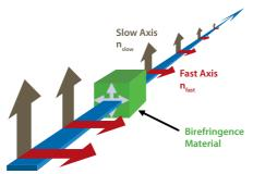
Figure 33: Propagation in a birefringence material
