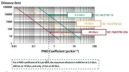
Figure 44. Maximum distant as a function of PMD coefficient and bit rate
