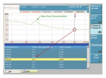
Figure 65. Measuring the attenuation profile with the T-BERD/MTS-8000
