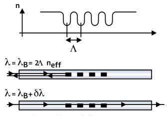
Figure 22. Schematic of a fiber Bragg grating
