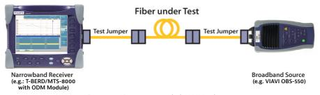
Figure 88. AP test setup with the VIAVI solution
