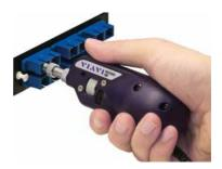
Figure 72. Bulkhead inspection
