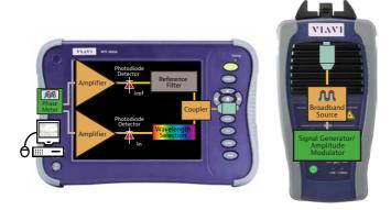
Figure 25. VIAVI Phase Shift solution: T-BERD®/MTS-6000A platform with ODM module and its associated broadband source
