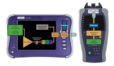
Figure 54. VIAVI Fixed Analyzer PMD module and the T-BERD/MTS-6000 platform
