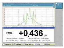
Figure 48. 100 km G.652 fiber link employing new fiber manufactured in 2002
