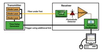
Figure 27: Typical schematic of the elements of the Pulse Delay method
