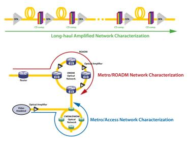
Figure 66. Example of route of tests for network characterization
