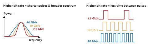
Figure 15. Effect of bit rate increase on pulse width and intervals
