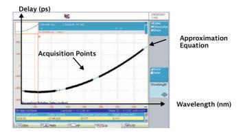
The CD is computed by calculating the slope of the group delay curve as a function of wavelength.
