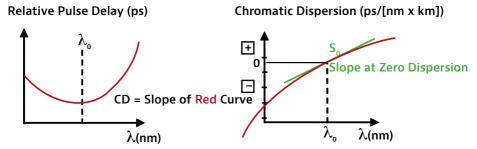
Figure 3. Examples of pulse delay, CD, and dispersion slope
