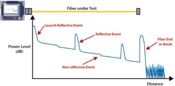
Figure 81. T-BERD/MTS-8000 with OTDR module and resulting trace
