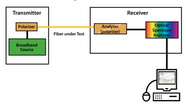
Figure 53. Typical schematic of the elements of the Fixed Analyzer method
