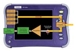
Figure 30: VIAVI Pulse Delay OTDR method in the T-BERD/MTS-6000 platform
