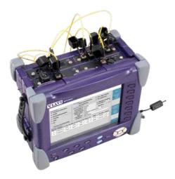
Figure 92. T-BERD/MTS-8000 configured with the MTAU module connected to the fiber characterization test module
