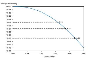
Figure 43. Outrage probability vs DGD<sub>Max</sub>/PMD
