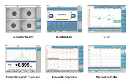
Figure 90. Summary of link characterization tests
