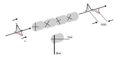
Figure 39: Strong mode coupling in telecommunications optical fiber
