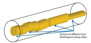
Figure 38: Fiber birefringence in an optical fiber link
