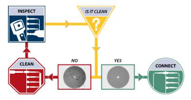
Figure 70. Connector inspection and cleaning steps
