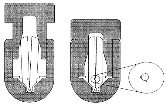
After preparation, the fibers are inserted into the Fibrlok II Splice element. The assembly tool is then used to close the the cap, forcing the clamping and locating surfaces against the fibers and aligning the fibers precisely and permanently in place.
