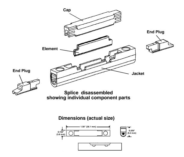
Cross-sectional view of open and actuated Fibrlok II Universal Optical Fiber Splice
