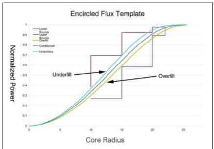
EF is a more sensitive way of defining power and it can be measured using imaging techniques. The vertical (Y) scale shows the total power from the core of the fiber up to a point on the radius (in microns), so when one gets to 25 microns, one measures all the power. The shape of the curve is chosen to emulate an idealized source that is between underfill and overfill conditions.
