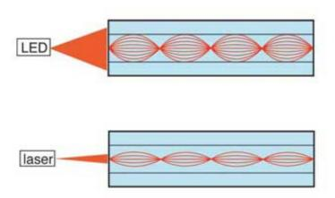
And, when testing cables designed for low speed LED transmitter type systems, using a LED source similar to the one used in the system and short launch cables may provide as accurate a measurement as is possible under more controlled circumstances, since the LED approximates the system source. For newer sytems using VCSEL sources, one should use at least a LED with a mandrel wrap (see below) or a commercially-available mode modifier.
