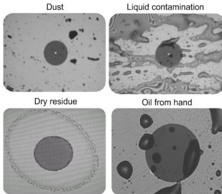
Figure 158: Appearance of various contaminants on a connector end face
