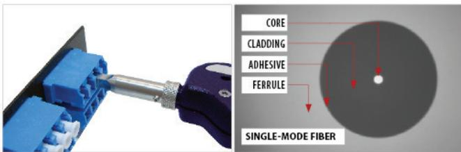
Figure 7. Microscope Inspection through the bulkhead/adaptor connector
