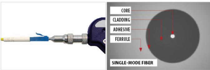
Figure 6. Patchcord microscope inspection
