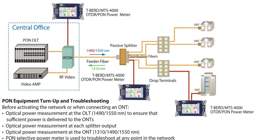
Figure 18. FTTH Network turn-up optical tools
