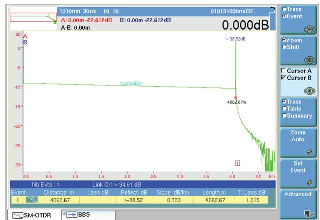
Figure 12. Feeder or distribution cable test only
