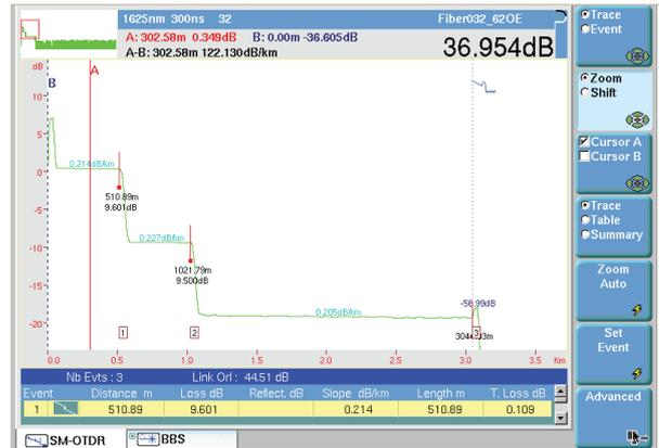
Figure 14. Cascaded splitter network test from ONT, without launch cable
