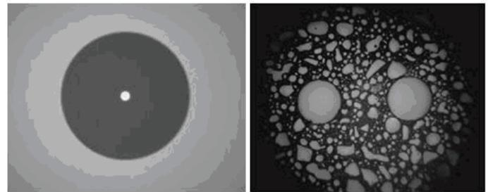
Figure 4. Microscopic views of clean connector end faces. Fiber Connector Inspect/Clean/Connect Process
