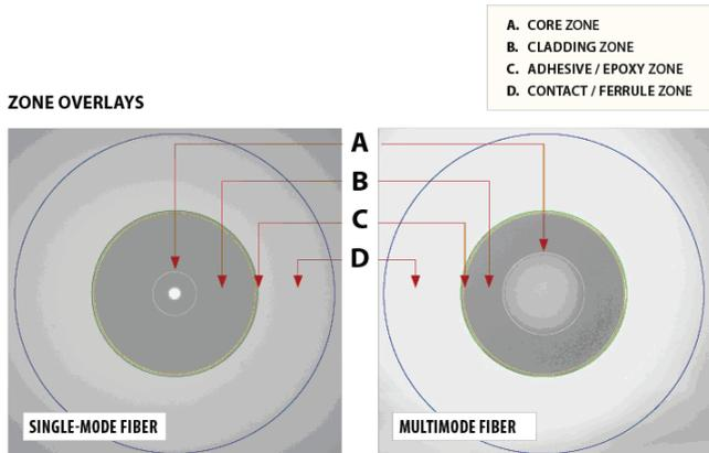
Figure 2. Fiber connector end face inspection zones
