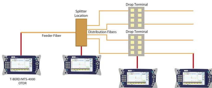
Figure 1. Possible access points for FTTH network qualification
