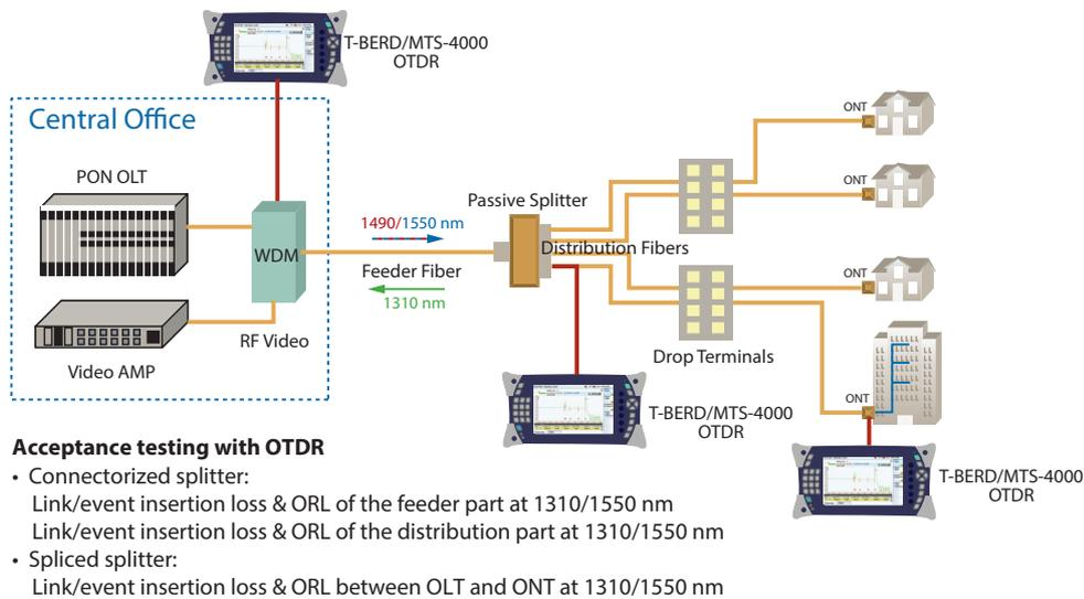
Figure 11. Qualifying a FTTH network with an OTDR
