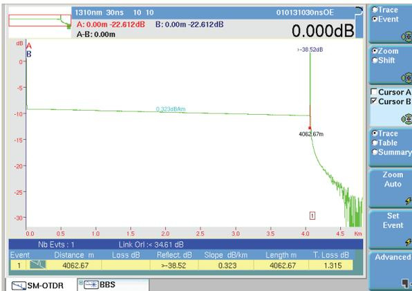
Figure 15. Feeder test only from the OLT to first splitter, without launch cable
