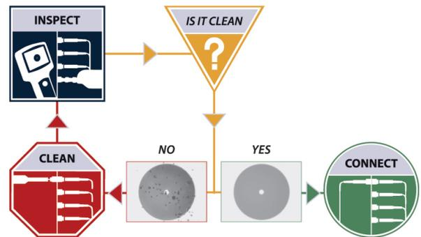
Figure 5. Optical connector Inspect/Clean/Connect Process
