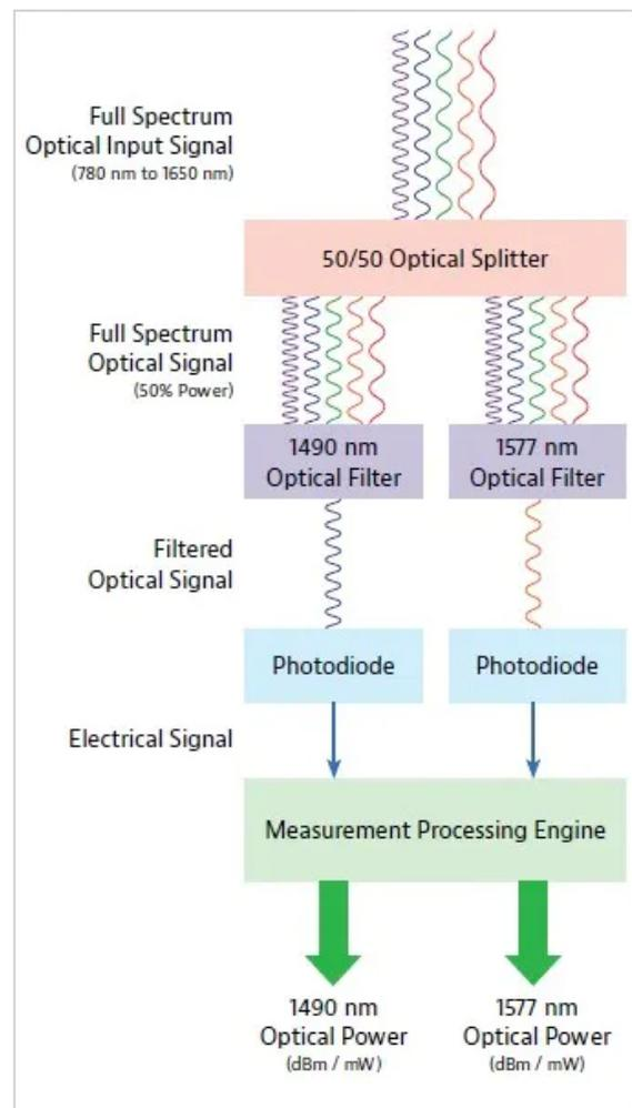
Figure 2. Selective optical power meter schematic.
