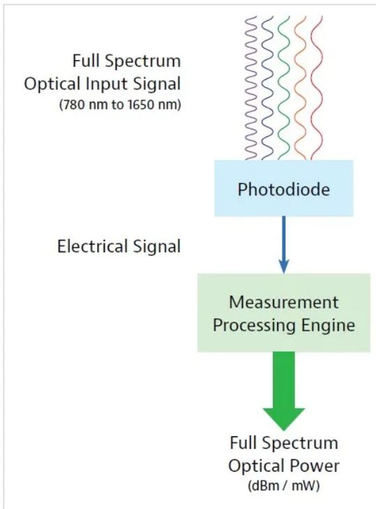
Figure 1. Broadband optical power meter schematic.
