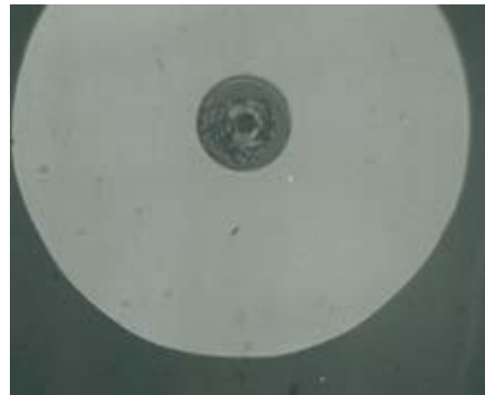
Figure 22 Dents from burning in the core area due to high power laser hitting end face contaminants
