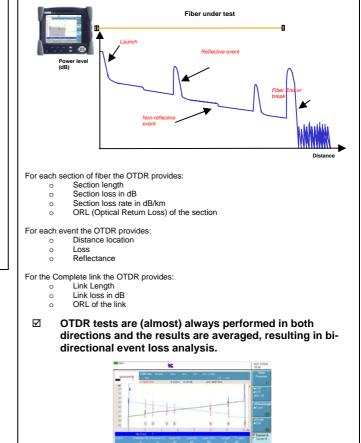
☑ The OTDR most commonly operates at 1310, 1550 and 1625 nm singlemode wavelength.
