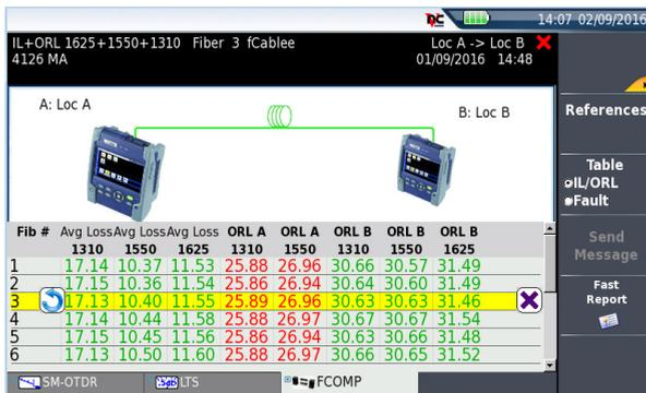
The **Cable View** allows to display results of multiple fibers:
