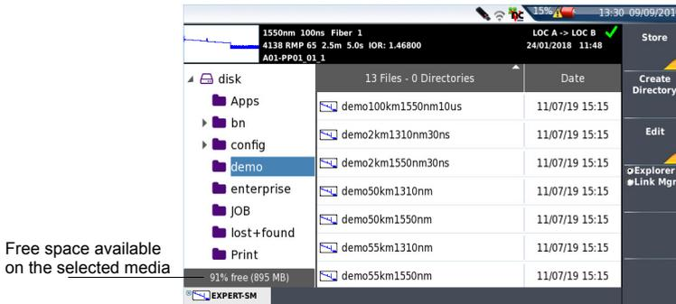
The direction keys can be used to move horizontally between the two parts and vertically within each zone.
