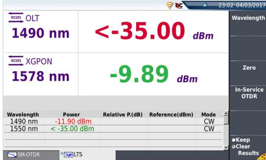
For each wavelength, the power value is displayed in green if it does not exceed the alarm thresholds defined in the setup menu, and in red if it exceeds the thresholds.
