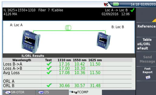
The Fiber View allows to display results of one fiber:
