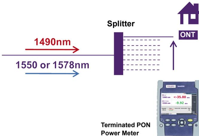
The SmartOTDR Terminated PON Power Meter measures simultaneously 1490 & 1550 nm or 1490 & 1578 nm downstream signals.
