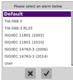
See [Table 1](#) and [Table 2](#) to get the values for each pre-defined alarm thresholds. The thresholds can be modified only in Expert mode and saved in a new configuration file.
