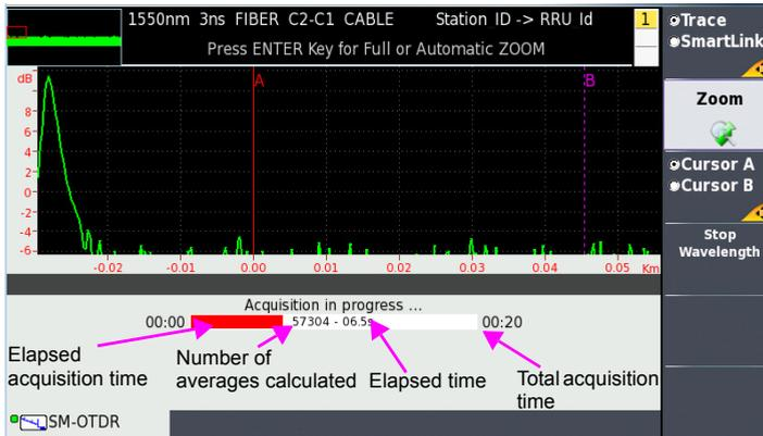
At the end of the acquisition, a beep is emitted, the trace is displayed and an automatic measurement is started.
