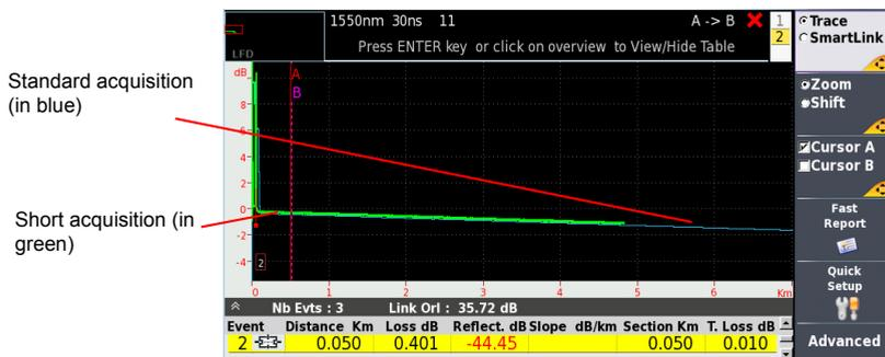
The short trace is the one resulting from the short acquisition and stops while the standard one continues until the end of measurement.
