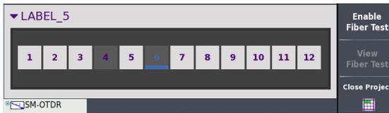
The disable fibers will be skipped while moving to the next fiber test.
