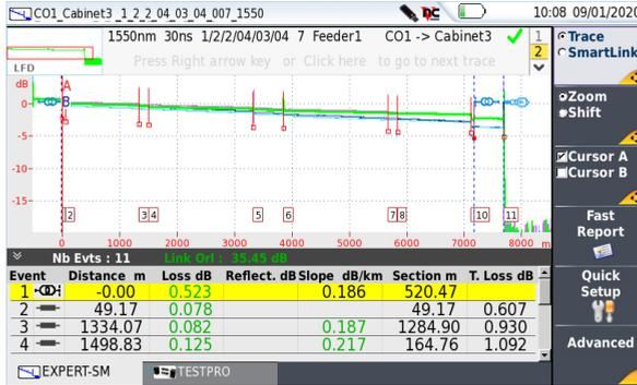
The results displayed in green or red are values for which a threshold has been defined: in green, the value does not exceed the thresholds defined in OTDR setup, in red it exceeds the thresholds. See “Configuring the Alarms parameters” on page 31.
