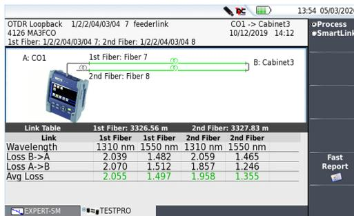
On the upper part, a graphical representation of the installation for the test is displayed, with the Identifier for each component (name of the location and of the loopback, fiber numbers...).
