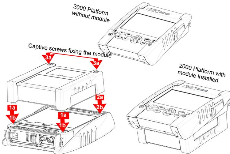
**Figure 3** Fixing the module to the 4000 V2 Base-Unit
