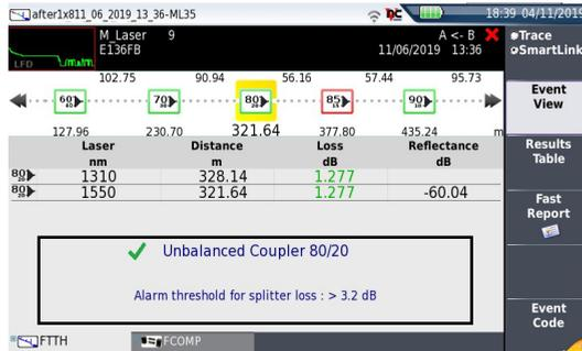
60 → The unbalanced or tapered optical splitters are identified with their respective ratio, and their loss value compared to the Alarm thresholds defined.
