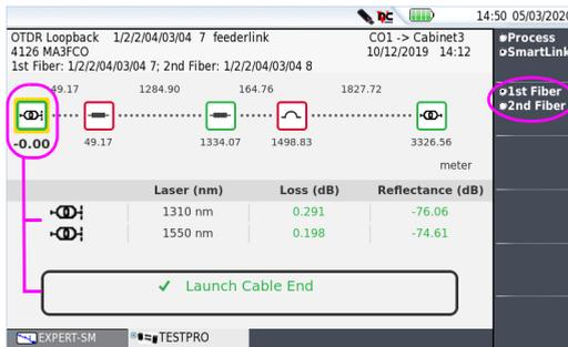
Click on one event on the graphical representation to display the loss and reflectance values for each wavelength, and the event description, at the bottom of the display.
