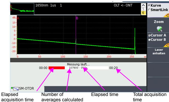
At the end of the acquisition, a beep is emitted, the trace is displayed and an automatic measurement is started.
