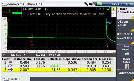
At the top of the table, a line shows the generic parameters of the fiber: numbers of events present, total ORL of the link and, in ExpertOTDR mode, reference trace icon (if trace is the reference trace - see ["Reference Trace function" on page 86](#)).
