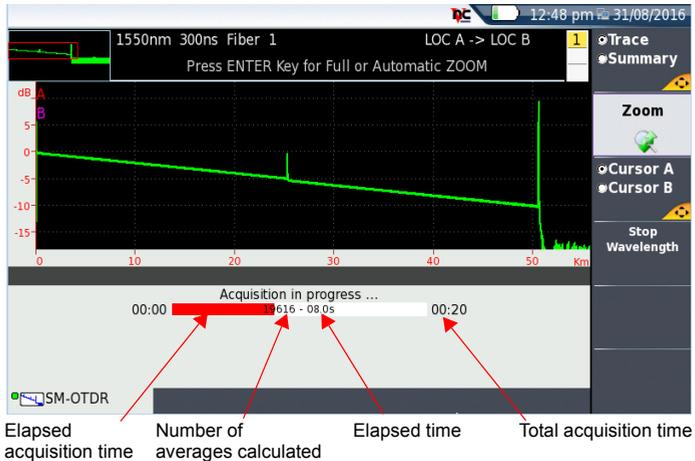
At the end of the acquisition, a beep is emitted, and the measurements are displayed, in SLM view, with a dialog box indicating the pass or fail verdict and asking if results must be saved.
