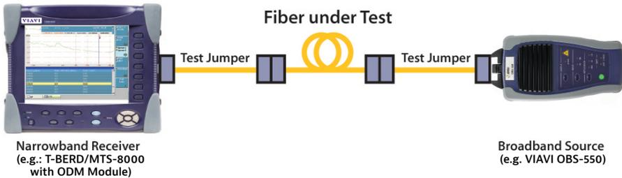
Figure 88. AP test setup with the VIAVI solution
