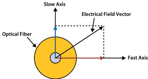
Figure 36: Signals transmitted through a birefringent fiber experience a slow and fast polarization mode. Therefore, a short signal pulse transmitted through a highly birefringent fiber may be decomposed into two orthogonally polarized pulses that travel at different speeds through the fiber, as shown schematically in Figure 37.
