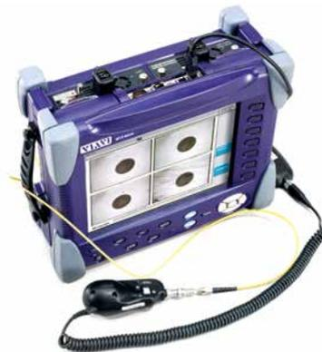
Figure 73. VIAVI T-BERD/MTS-8000 platform and video scope combination
