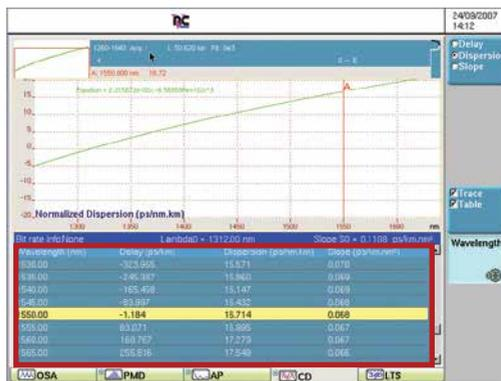
Figure 85. CD results with the VIAVI Phase Shift method (ODM module)
