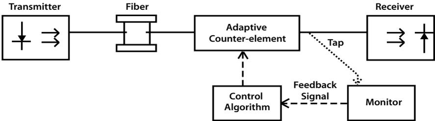
Figure 49. Schematic diagram of an optical PMD compensator
