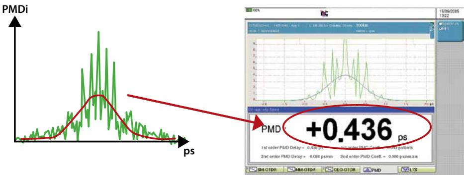
Figure 87. PMD measurement display with the VIAVI Fixed Analyzer method in the T-BERD/MTS platform
