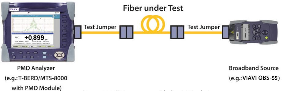
Figure 86. PMD test setup with the VIAVI solution
