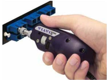
Figure 72. Bulkhead inspection
