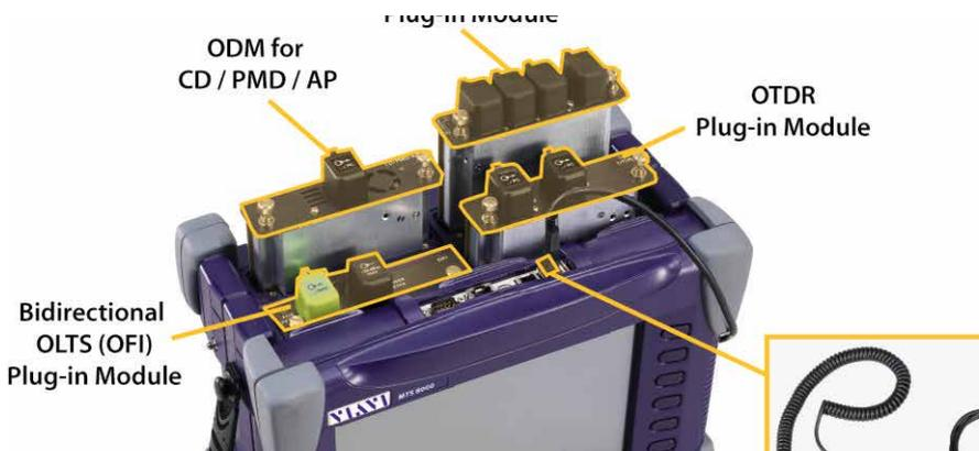
Figure 68. VIAVI T-BERD/MTS-8000 with its plug-in modules and accessories for fiber characterization
