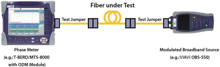
Figure 84. CD test setup with the VIAVI solution
