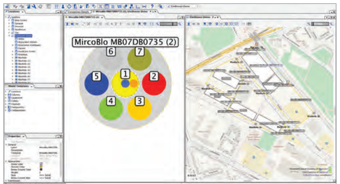
CMS allows visibility of campus level networking, including detailed management conventional and air-blown fibre.
