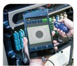
Inspect Automated pass/fail fiber inspection with a P5000i microscope
