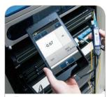
Test Measure optical power with an MP-Series optical power meter
