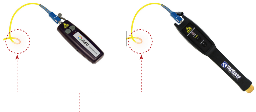
Red illumination indicating fiber damage/bend
