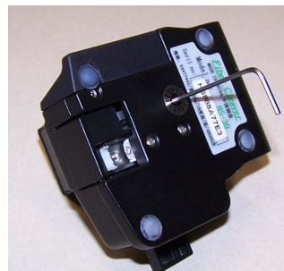
5.3 Access the blade arm position screw underneath the tool. Turn the screw clockwise 1 index position (1/12th of a turn) with 1.5mm allen wrench to raise the arm and blade. More than two index moves will raise the blade too much.
