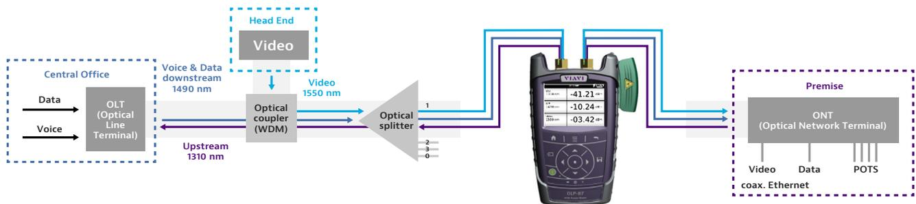
In addition the new generation of PON testers can use PON-ID information and G-PON data analysis to determine ONU/ONT service activation status, allowing techs to check if an ONU/ONT is provisioned correctly with the OLT and to verify an ONU/ONT is routed to or connected to the correct OLT port. Plus checking for any rogue or alien ONU/ONT devices potentially disrupting service to other customers.
