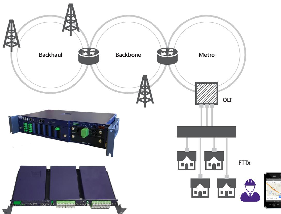
ONMSi offers a comprehensive fiber monitoring solution: it supports metro, core, access, and PON networks.
