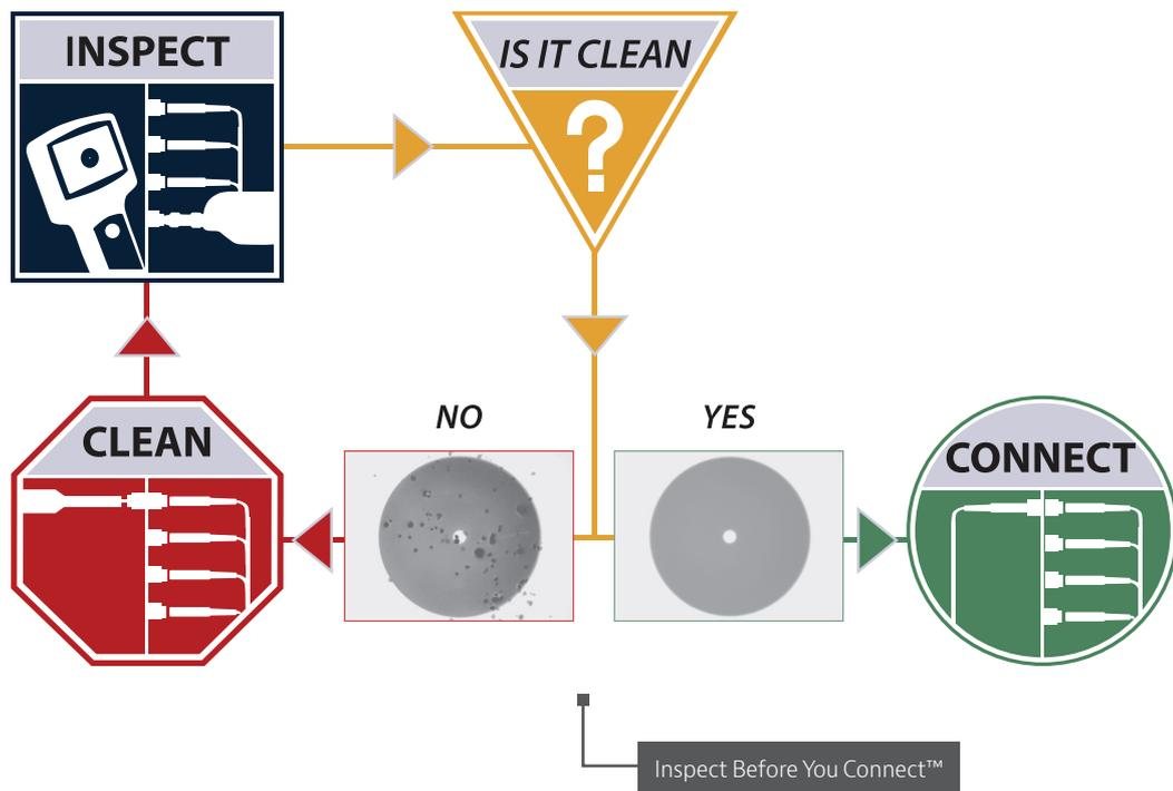
VIAMI offers a comprehensive product portfolio for inspecting every fiber connector and application in your network. Consistent use of the “Inspect Before You Connect” (IBYC) model ensures that proactive inspection is performed correctly every time prior to mating. This eliminates the installation of dirty or damaged fibers into the network and optimizes network performance.
